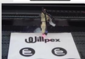
CÁMARA (CCD) PARA CORTE CONTORNO GRABADORA LÁSER WILLPEX 1390
